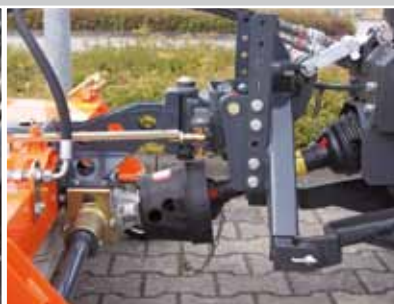
PTO-drive for 540 up to 2100 rpm
