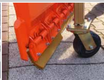
PU coated (standard) anti-icing spring flap segments
