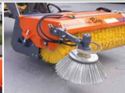
Fully adjustable hydraulic side brush (50% PP / 50% wire)
