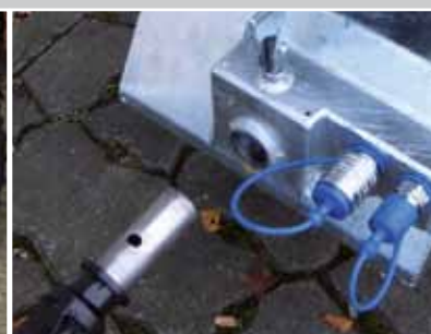
Hitch system and double-acting hydraulic connector (standard)
