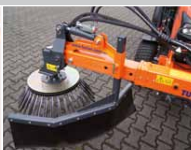
Telescopic, with hydr. inclination adjustment
