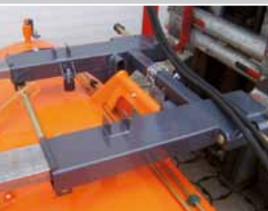
Hitch system with 3D levelling (standard)
