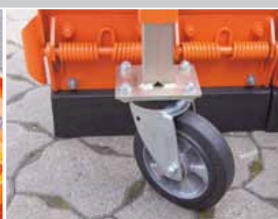
Spring flap segments (anti-icing)
