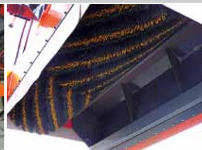
Special V-brush for sticky and fine dirt
