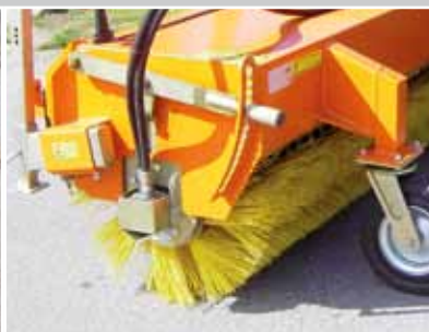
2 strong, internal motors for driving the main brush
