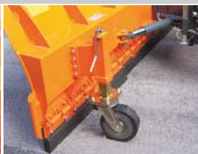
Infinitely height adjustable wheels
