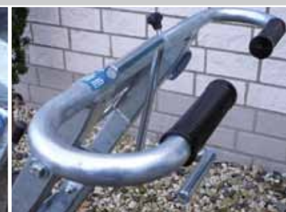
Height adjustable guiding-rod incl. forward/backwards gear
