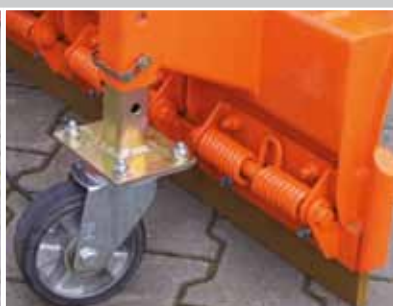
Spring flap segments (anti-icing)
