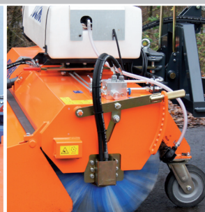
Adjusting-lever system with optimized sweeping-angle
